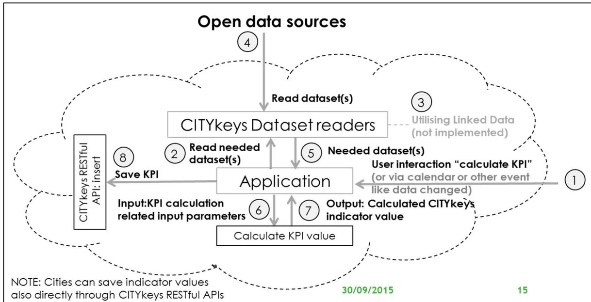
Figure 8. Main concept of the CITYkeys automatic data reading.
